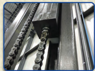
Counterweight system for smooth operation without vibration, resulting in a safer operation
