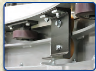
Horizontal and vertical ring guiding by self aligning and maintenance free polyurethane wheels
